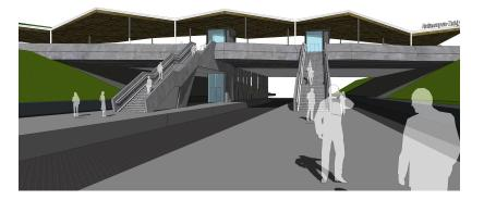
The existing accesses (concrete stairs and escalators) to the platforms in Antwerp South station will be demolished and replaced by a bicycle lift and precast concrete stairs.
